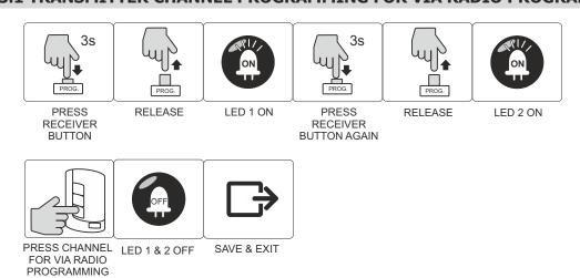
\*Note: When enter into programming of a programming via radio channel, the relay output will be active.
