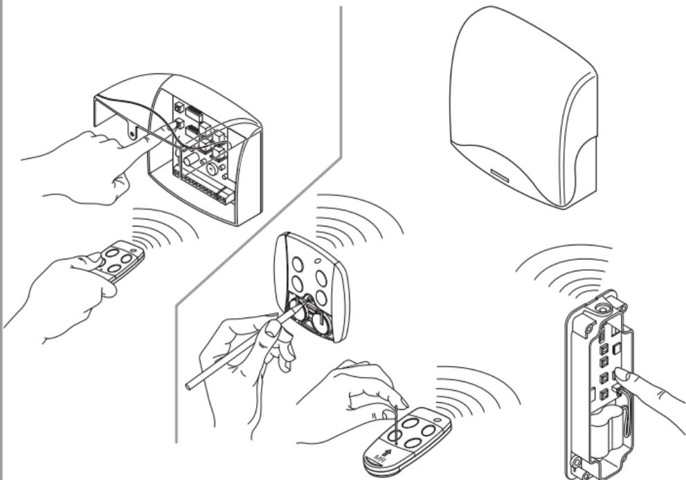
RICEVITORE IN CASSETTA - OUTDOOR RECEIVER - RÉCEPTEUR AVEC BOÎTIER
