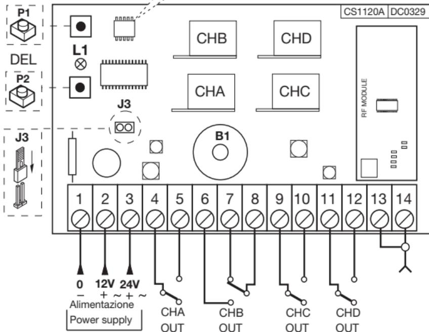
**RICEVITORE A SCHEDA AD INNESTO DIRETTO - SLOT-IN RECEIVER CARD**
